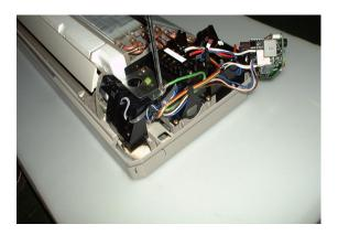
③ Remove the screws (3) attaching the electrical component box, and remove the box from the frame by pressing the tabs at the back of the box.
